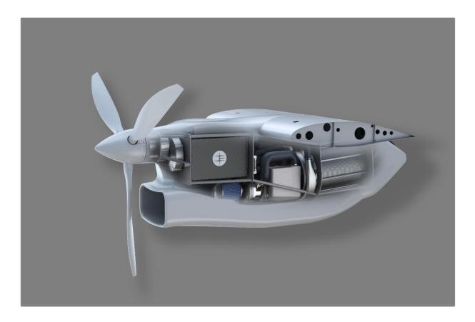
Intelligent Energy launch breakthrough IE-FLIGHT hydrogen fuel cell system products to power subregional and regional flights
